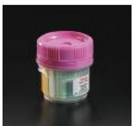
As a cassette holder, the 40 ml HistoTainer™ containing 20 ml of 10% Formalin, is the ideal size container to transport up to four tissue samples pre-inserted in processing/embedding cassettes.
