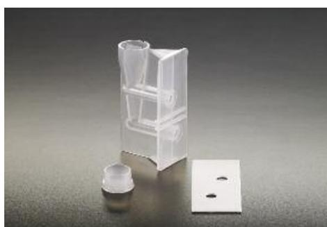
The Simport Double CytoSep™ Cytology Funnel with disposable sample chamber allows for two samples to be run simultaneously on a single slide and is ideal for immunohistochemistry work. The Double CytoSep™ Cytology Funnel provides a cell deposition area of 6 mm (28 mm squared) for sample volumes of up to 0.5 ml. The filter card comes pre-attached. Cap is included. No need to use a different stainless steel slide clip. Each component is also available separately.
